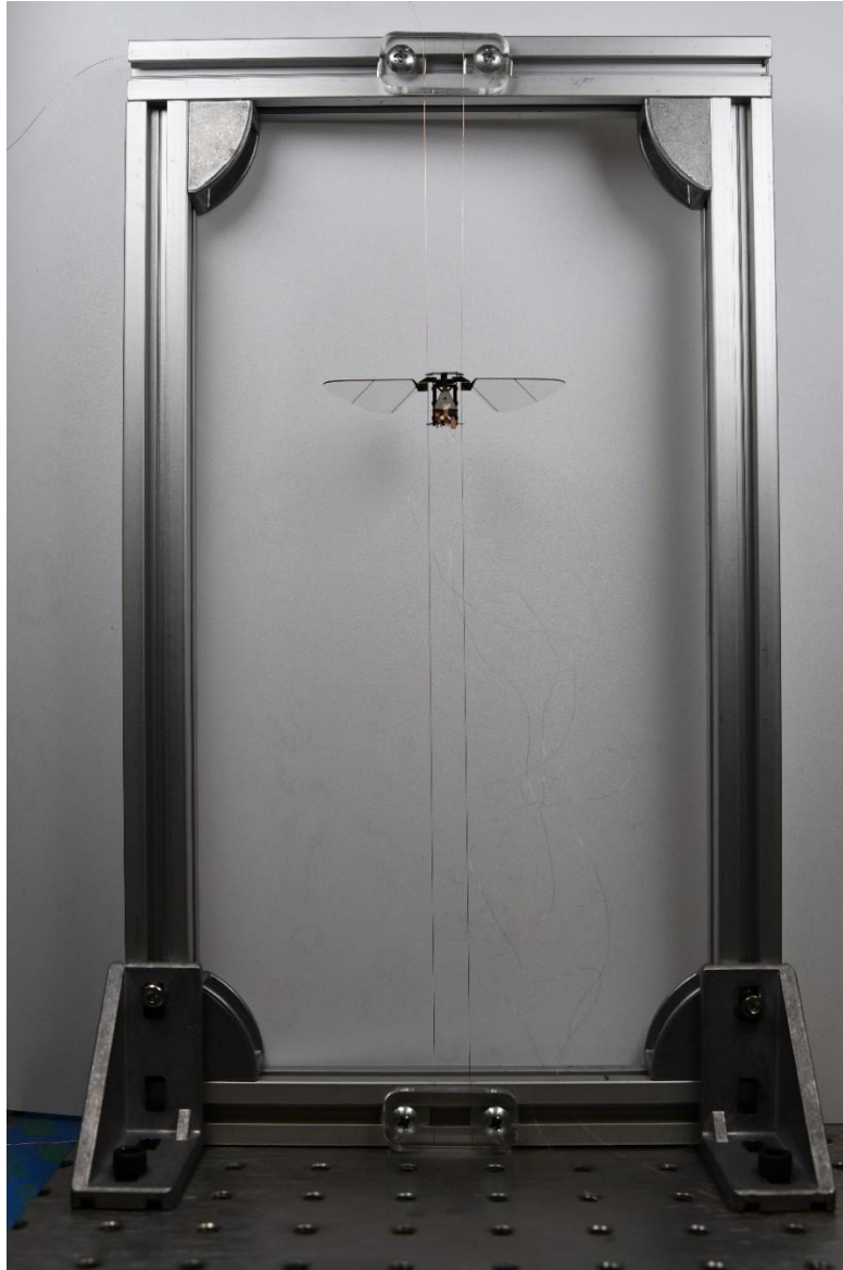
Figure 13. The Upscaled RoboBee Sits On a Vertical Rail System With Copper Wires Acting as Low Friction Guides
