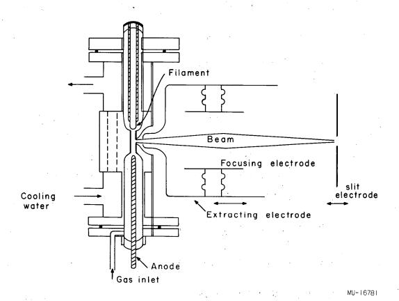
Figure 1. Details of the ion source of the isotope separator.
