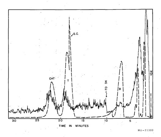
Figure 3. Mass (dashed line) and radioactivity (full line) record of the gas-chromatographic separation of the products of the lucture irradiation of benzene.
