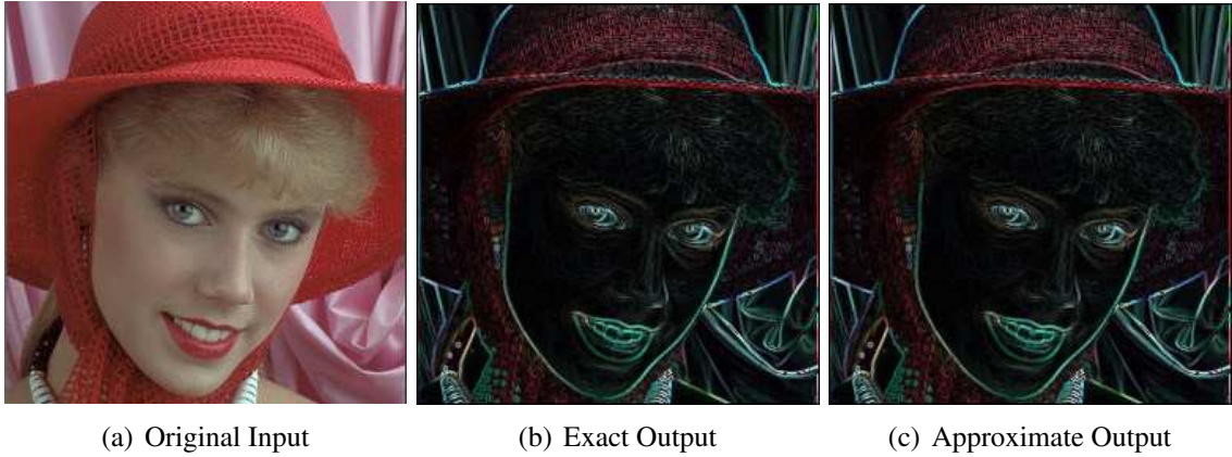
Figure 2.3: (a) Original input image. (b) Error-free exact Sobel filter output with PSNR = inf. (c) Error-injected approximate Sobel filter with PSNR = 30dB.
