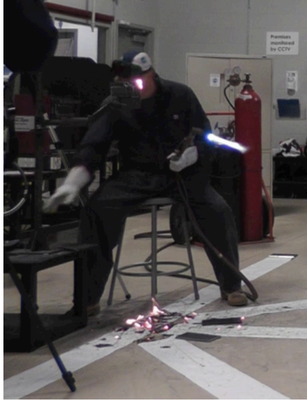
Figure 1.1: Thermal Paper Set Alight by Oxyacetylene Slag [30].
