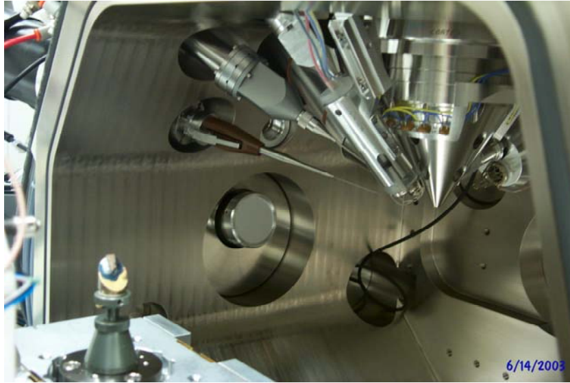
Figure 2. FIB Sample chamber with sample mounted on 45 deg stage
