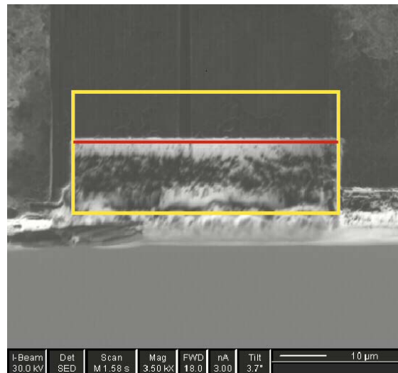
Figure 4. View from the ion beam direction of sample surface A during milling. The milling boundary is defined by the white rectangle and the most recent surface exposed is marked by the middle horizontal segment
