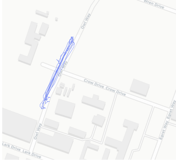
Figure 4.13: Top-down view of the INS pose estimates overlaid onto a map for all the alarm encounters. The blue lines should be within the bounds of the road, Owl Way, but there is a drift of the estimates over time.
