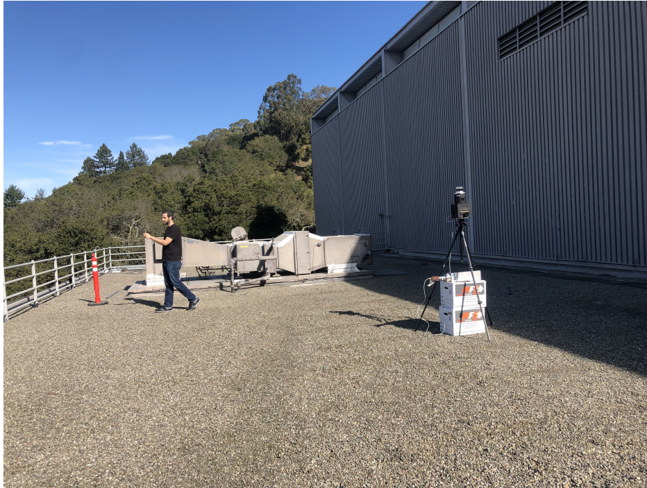
Figure 3.5: A person walking 5 m at closest approach in front of the static contextual system carrying a ^{137}\text{Cs} source.
