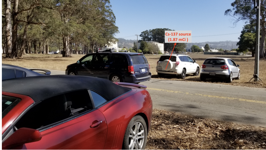
Figure 4.2: A degenerate scenario where LEMURS drove straight down the center of the road with cars parked on either side of the road. A 1.87 mCi ^{137}\text{Cs} source inside of 2 cm Pb shielding was placed in the trunk of a vehicle.
