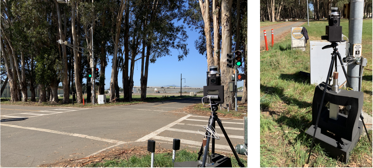
Figure 3.9: The contextual system, co-located with a NaI(Tl) detector, at the corner of an intersection at the University of California’s Richmond Field Station (RFS).
