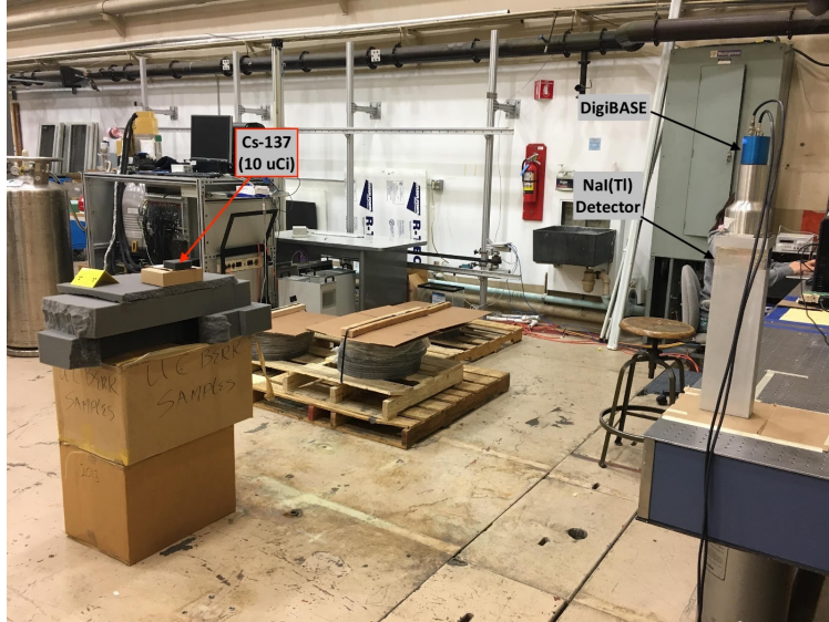
Figure 3.2: Experimental setup of a NaI(Tl) bar and ^{137}\text{Cs} source to find the photopeak efficiency of the detector at different source angles.
