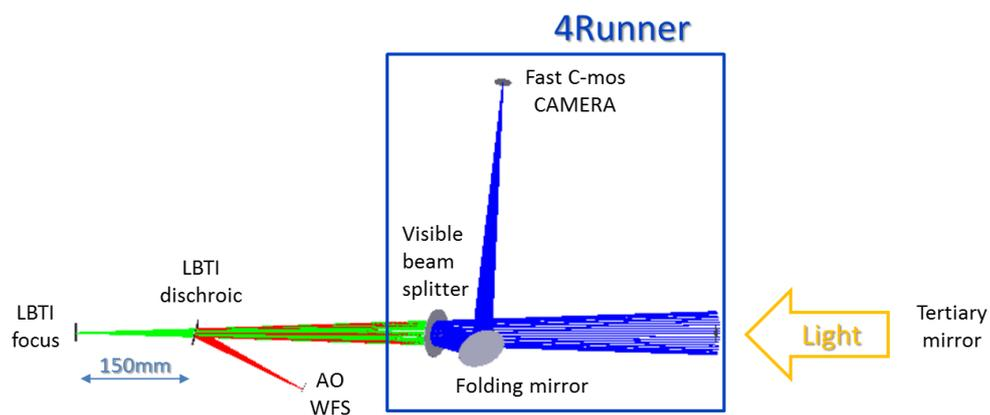
Figure 4. Zemax layout of the 4Runner's optical configuration.
