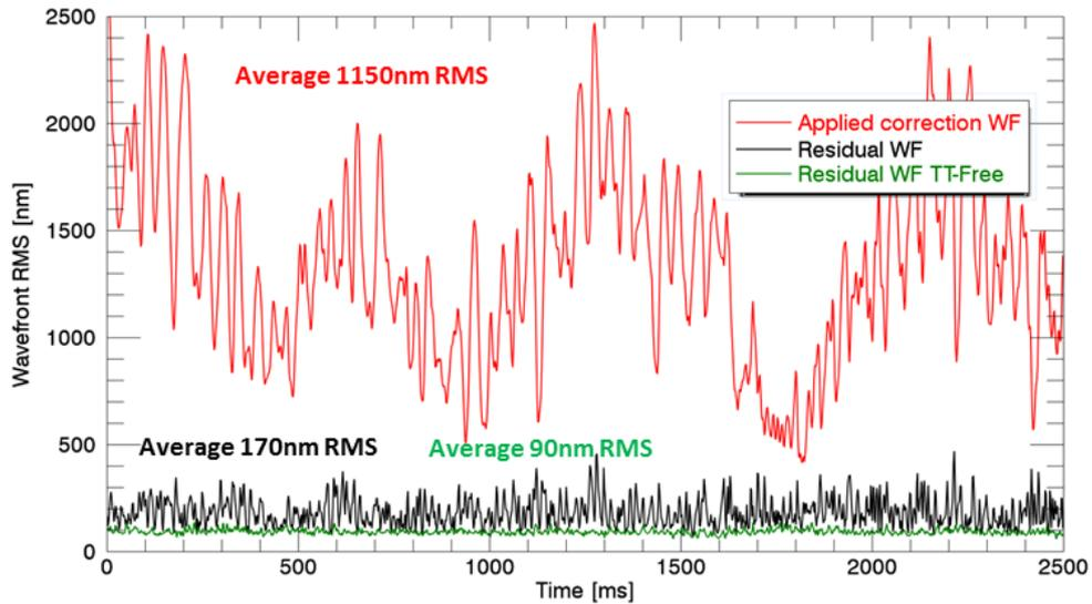
**Figure 6.** The plot represents the temporal behavior of the applied correction (red), the residual (black) wavefront error estimated by the WFS and the same value without considering the tip-tilt residuals. These values are computed from on-sky measurement as described in the body text.
