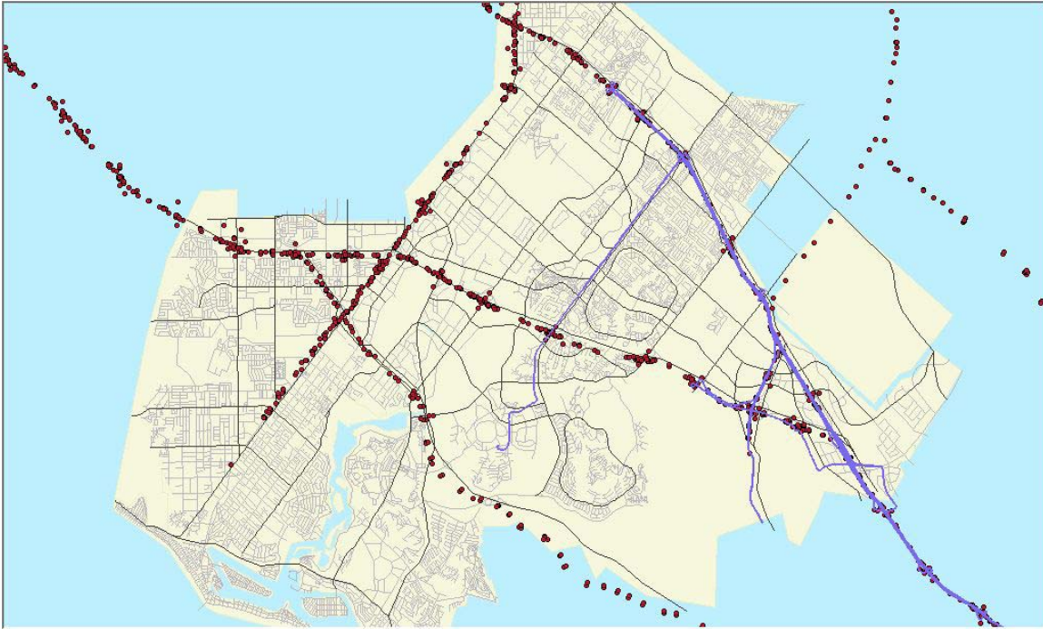
Figure 6. Sample Tracings (red dots are Caltrans loop detector stations)
