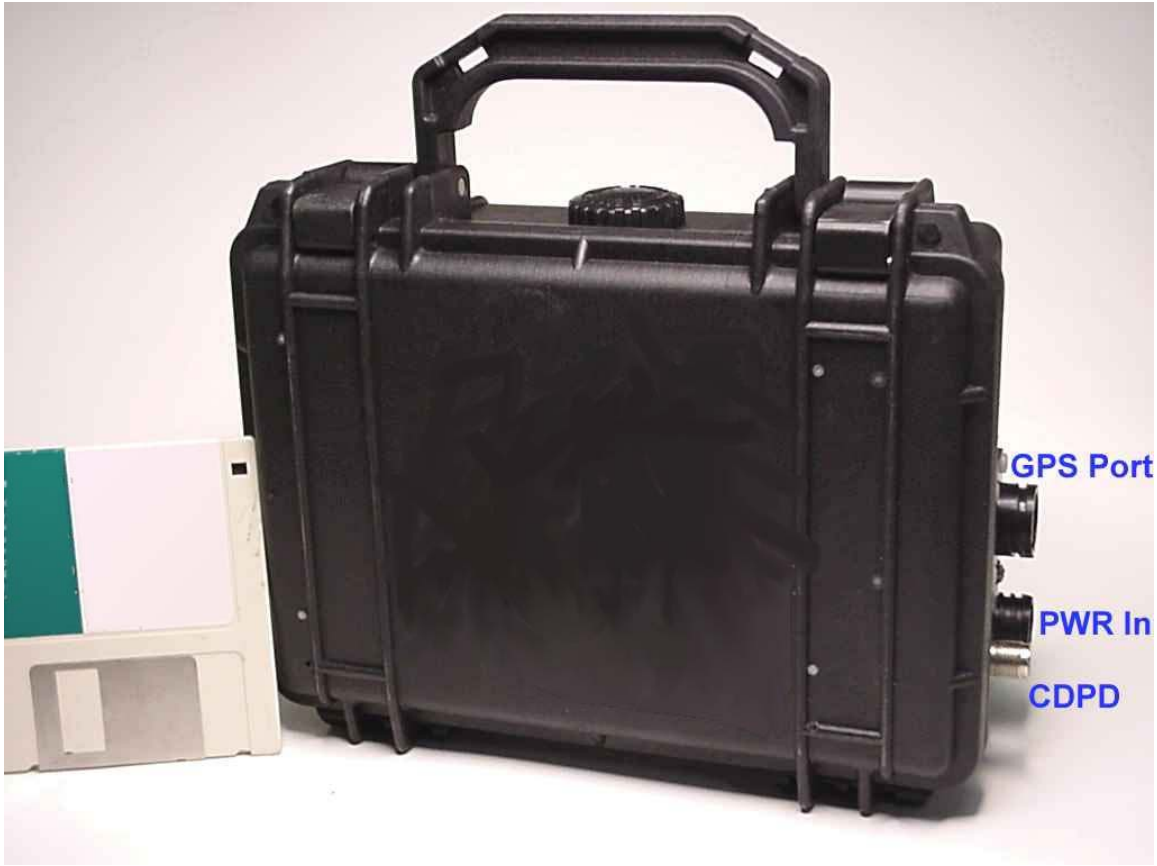
Figure 1. Prototype EDCU in R100 Case (exterior view)
