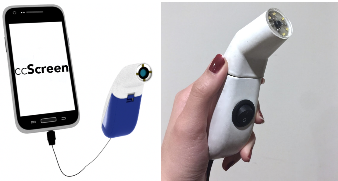
Figure 5-7. ccScreen v2 schematic [left] and 3D printed prototype [right]. Source: InVia.
