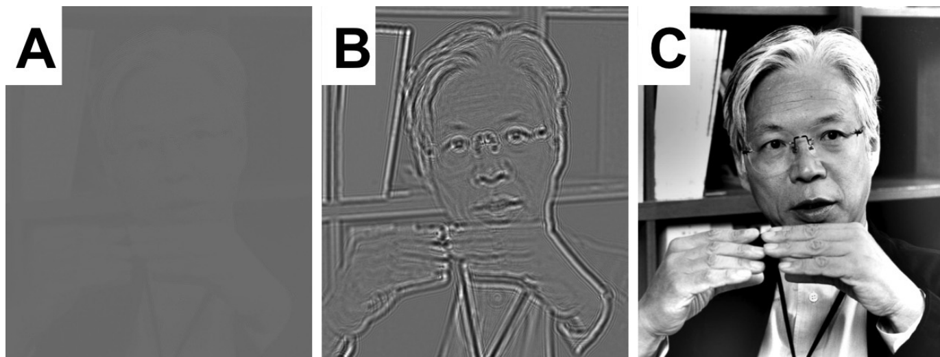
Figure 1. Simulations showing how a quarter-wave phase plate improves the contrast of in-focus images. In these simulations the intensity of the beam (which can be made of light or electrons) remains the same everywhere it passes through the “transparent” object; however, the phase changes significantly where the beam passes through different parts of the object. (A) A perfectly focused, bright-field image has almost no contrast because it can only show variations in the transmitted intensity. (B) A defocused image is able to capture at least a small part of the changes in the phase, so the contrast is better and the object can be seen. (C) Zernike realized that changing the phase of the unscattered portion of the transmitted wave (that is, the part that was not deflected when the wave passed through the object) by 90 degrees greatly improved the quality of the image. The scientist in the photograph is Professor Kuniaki Nagayama, who has played a seminal role in the development of phase plates for use in the transmission electron microscope. Image credit: Dr. Radostin Danev.
