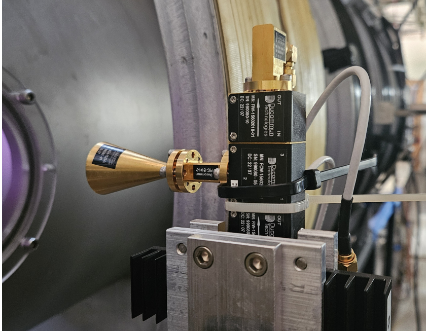
Figure 15: Photo of the homodyne Michelson interferometer.
