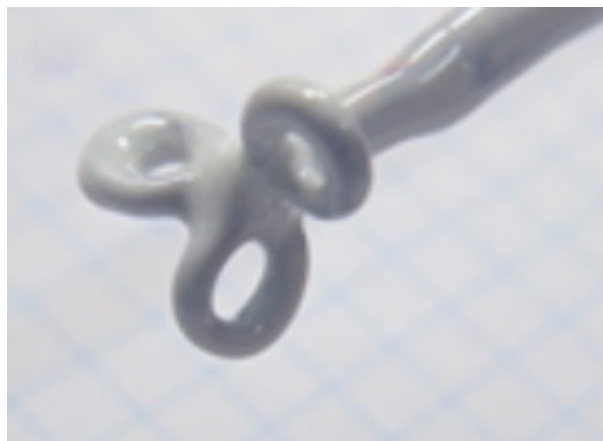
Figure 12: Probe tip of the three-axis 3.4 mm diameter Bdot probe, shielded with epoxy. Distance between the center of each loop is 5 mm
