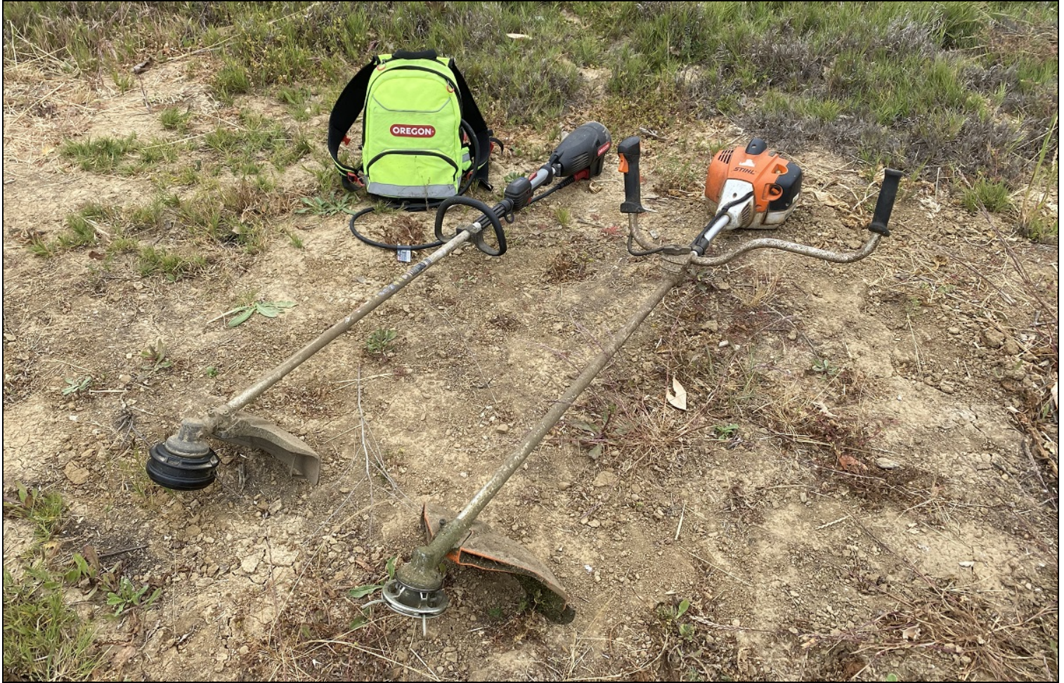
One of CCBER's new battery powered string trimmers (left) next to a gas powered trimmer (right) for comparison.
