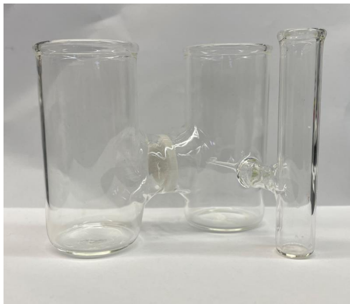
Figure 3.40: Glass frit separated H-Cell
