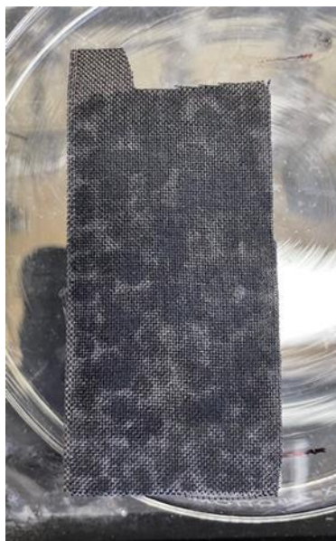
Figure 3.39: Example of a 34 cm 2 CF|CNT| PO Cb electrode
