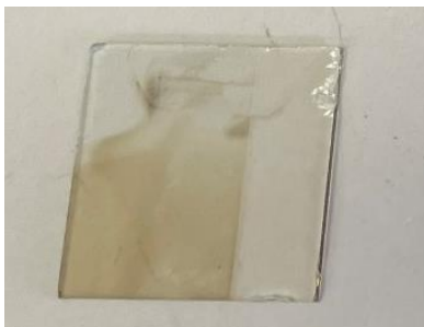
Figure 3.15: ITO electrode after CVs in aqueous solutions
