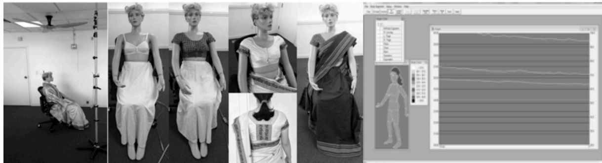
Figure 2. (Left to right) The test conditions of the climate chamber showing the data-logger setup; manikin with petticoat, panty, bra and bodice; a rear view of a sari and bodice on a human subject; manikin in a sari ensemble; the manikin control screen
