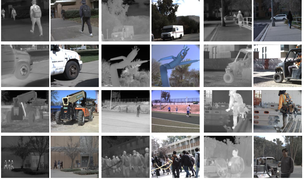
Figure 3.3: Dataset Snapshot. The visualization above shows a snapshot of the diverse set of images captured by our synchronized optical setup. We captured indoor scenes, outdoor scenes, scenes with moving humans, with moving vehicles, day time, and night time. Our dataset offers a significant contribution to computer vision in the thermal wavelengths.
