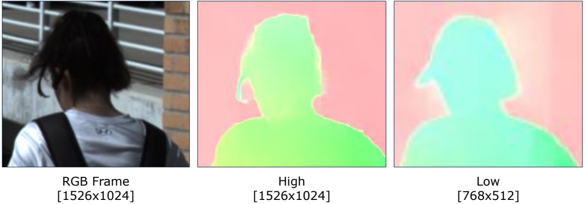
Figure 3.2: Resolution influence. Optical flow visualizations show the loss of detail in downsampled, lower-resolution input compared to the original higher-resolution input.
