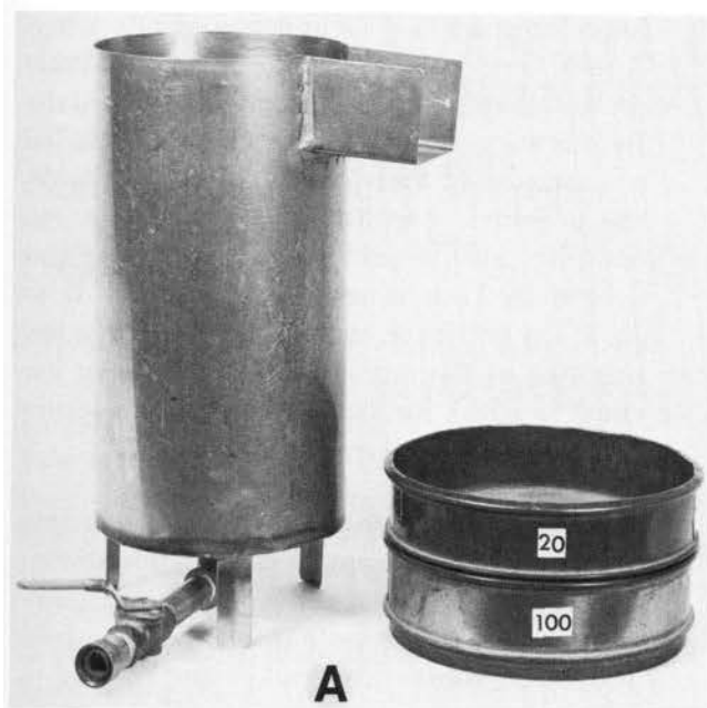
Fig. 17. Heterodera schachtii cyst extraction by flotation can and sieves. A. Apparatus used. B. Diagrammatic representation of extraction process. (A.—courtesy Herb Quick.)
