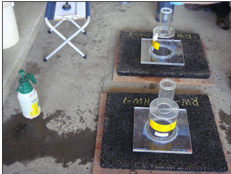
Figure 7.1: Permeability testing on compacted slabs.
