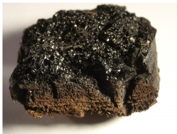
Figure 8. A carbon sample from a Carolina Bay that varies from the shiny, melted appearance of glass-like carbon at the top to Yellow Pine on the
