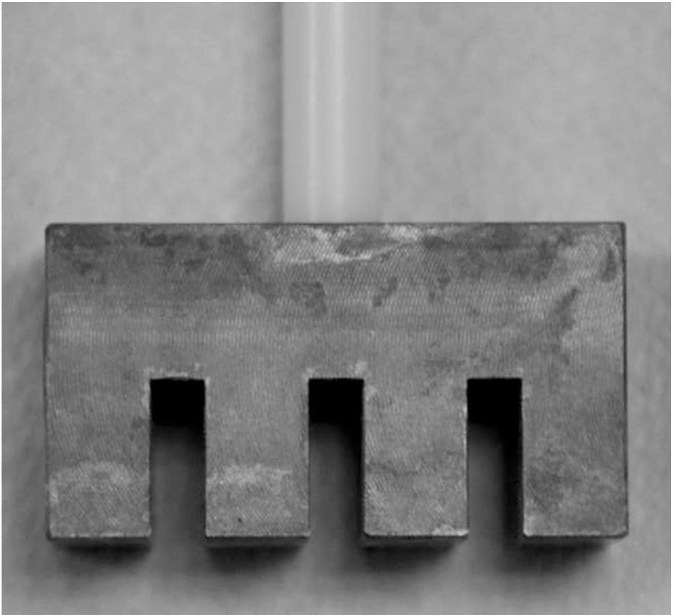
Figure 1. Brass comb used for burn induction.
