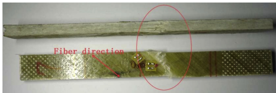
Fig. 8. Failure mode of in-plane shear specimen.
