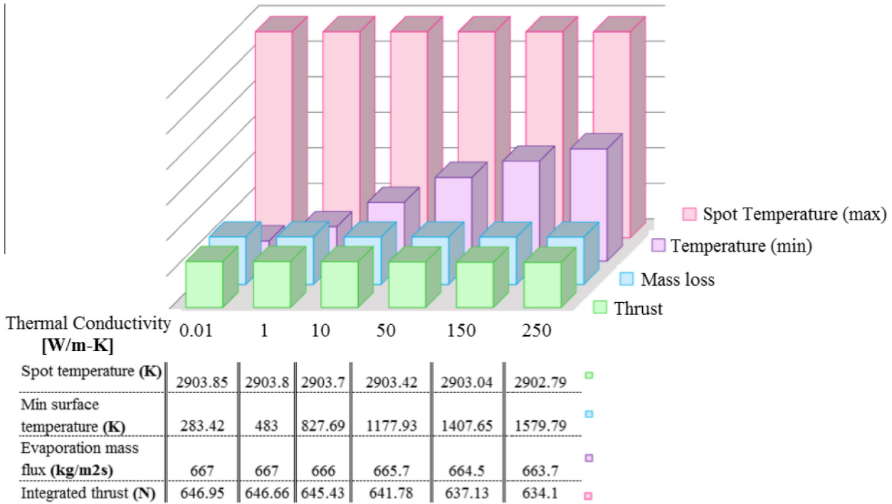
Fig. 24. Extreme values inputs of thermal conductivity set to 0.01–250 W/m K for SiO 2 – using 1 MW laser power, spot diameter is 60 mm, with sigma 10 mm, in this case for a 2 m diameter asteroid.
