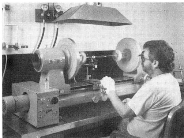
Figure 1. High-intensity discharge surface wave lamp is formed and extruded on high-temperature glass lathe. (CBB 901-343)
