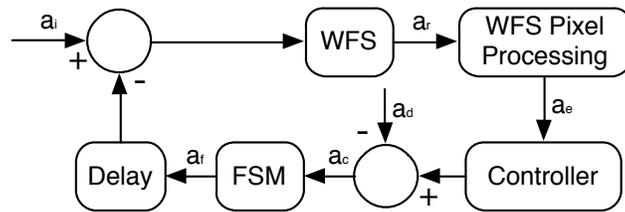
Figure 2: LGS beam uplink control
