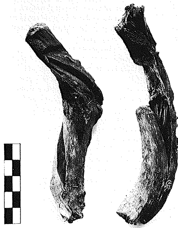
FIGURE 5.43 Effect of air drying on wet wood from Greece: A, when excavated; B, 32 years later.
