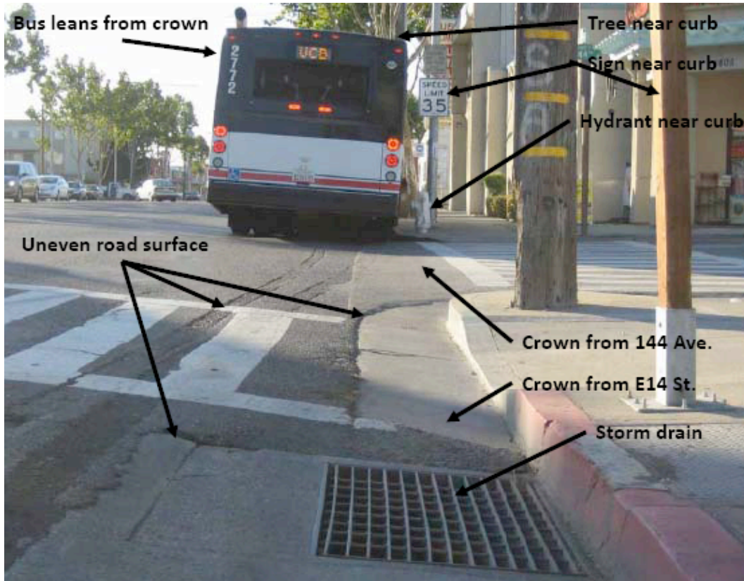
Figure 32 Station #2 Docking Precision Performance (Uneven Road Surfaces)
