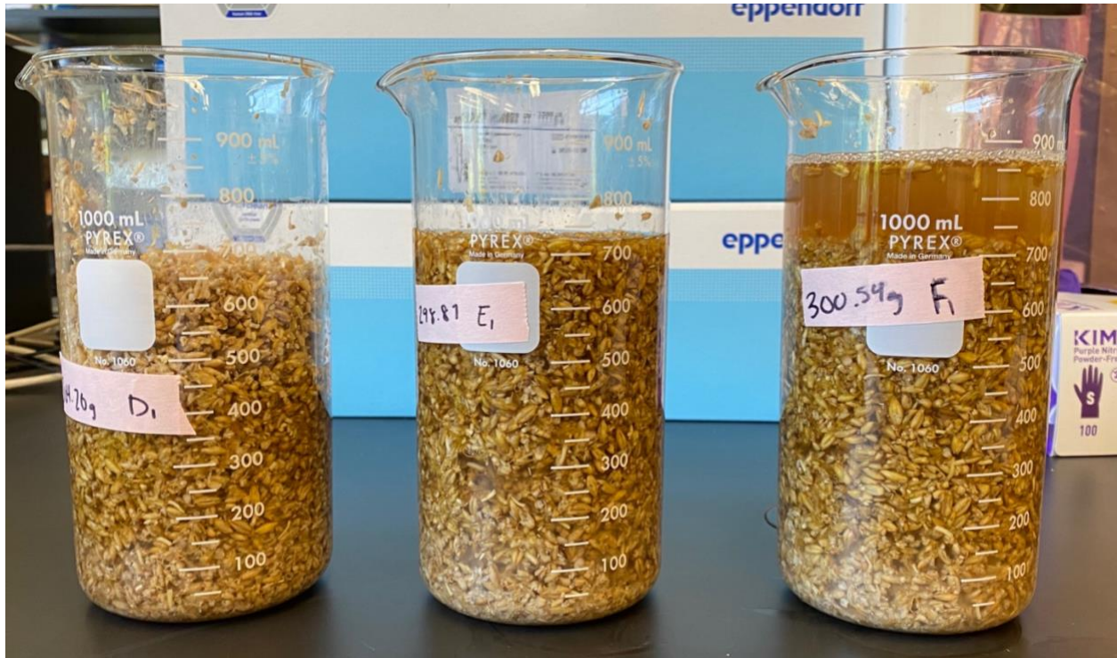
Image Description: three samples of brewers spent grains soaked in caustic, all weigh 400 g.
