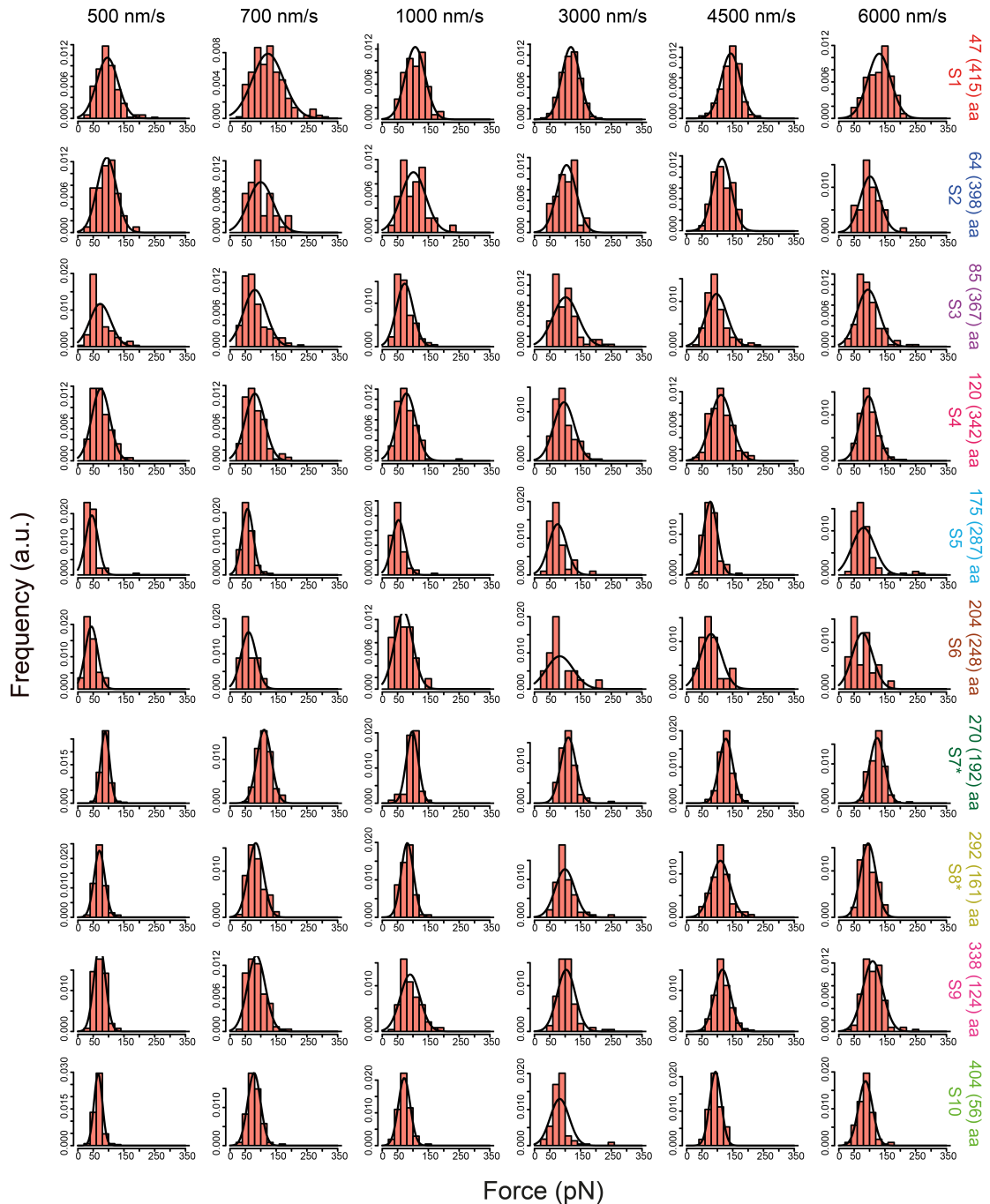
Fig. S10. Forces of unfolding force peaks recorded upon unfolding of mutant C154G LacY in the presence of substrate ( \alpha NPG). Histograms show the force distribution of every unfolding force peak recorded for six different pulling velocities (500, 700, 1000, 3000, 4500, and 6000 nm/s). Colored numbers on the right side give mean contour lengths (in aa) obtained by fitting the force peak classes from contour length histograms (comp. Fig. 6), numbers in parentheses give the amino acid position at which a stable structural segment starts in LacY. The bin size of all histograms is 20 pN. Dark blue lines are Gaussian fits of force distributions. The DFS data is obtained analyzing the FD curves shown in Fig. S7.
