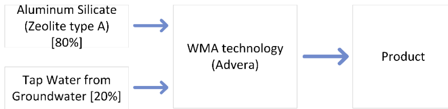
Figure 3.3: Process diagram used for modeling WMA technology—Advera.
