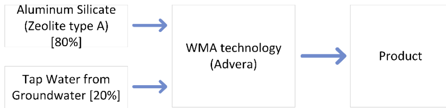
Figure 3.3: Process diagram used for modeling WMA technology—Advera.
