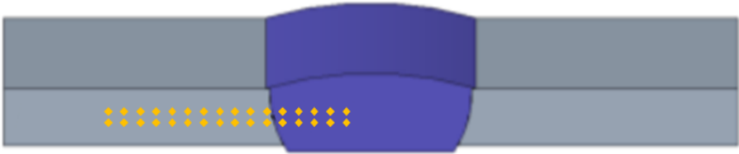
Figure 38 Schematic of microhardness measurement
