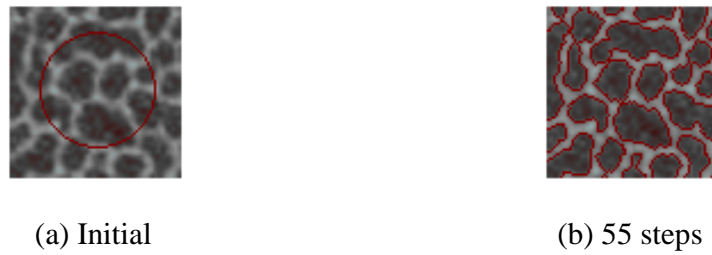
Figure 6-8 Interface identification of a microstructure by RKCM; (a) Initial trial interface; (b) Final evolved interface
