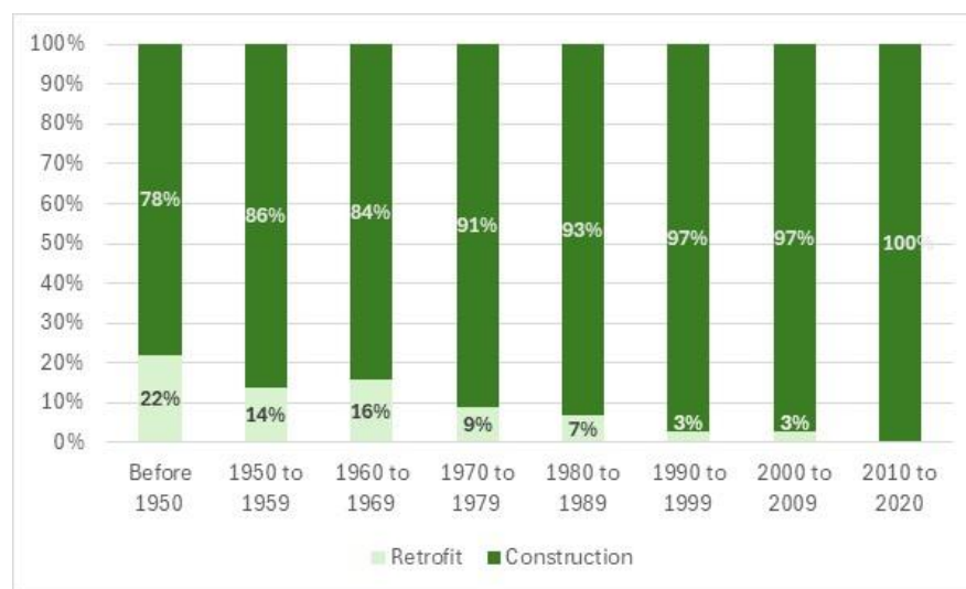
Figure 1 Commercial building installed fenestration by building vintage (“Construction” refers to fenestration remains from the original construction).
