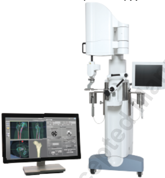
Figure 1: The TSolution One system for Total Hip Arthroplasty (THINK Surgical, Fremont, California).
