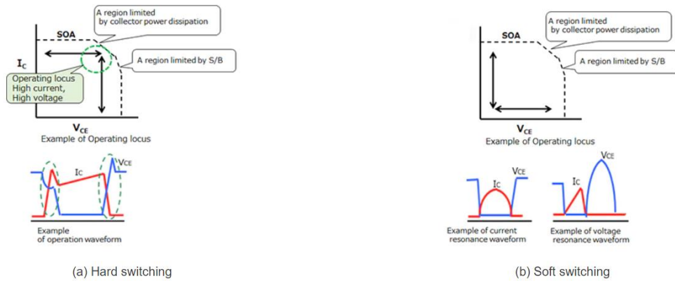
Figure 44. Characteristics of Hard-Switching versus Soft-Switching [17]
