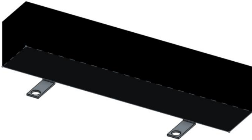
Figure 43. Physical Layout of Custom Capacitor for ‘XM3’ Family Inverter Design
