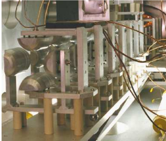
Electrostatic quadrupole lenses for beam set-up
