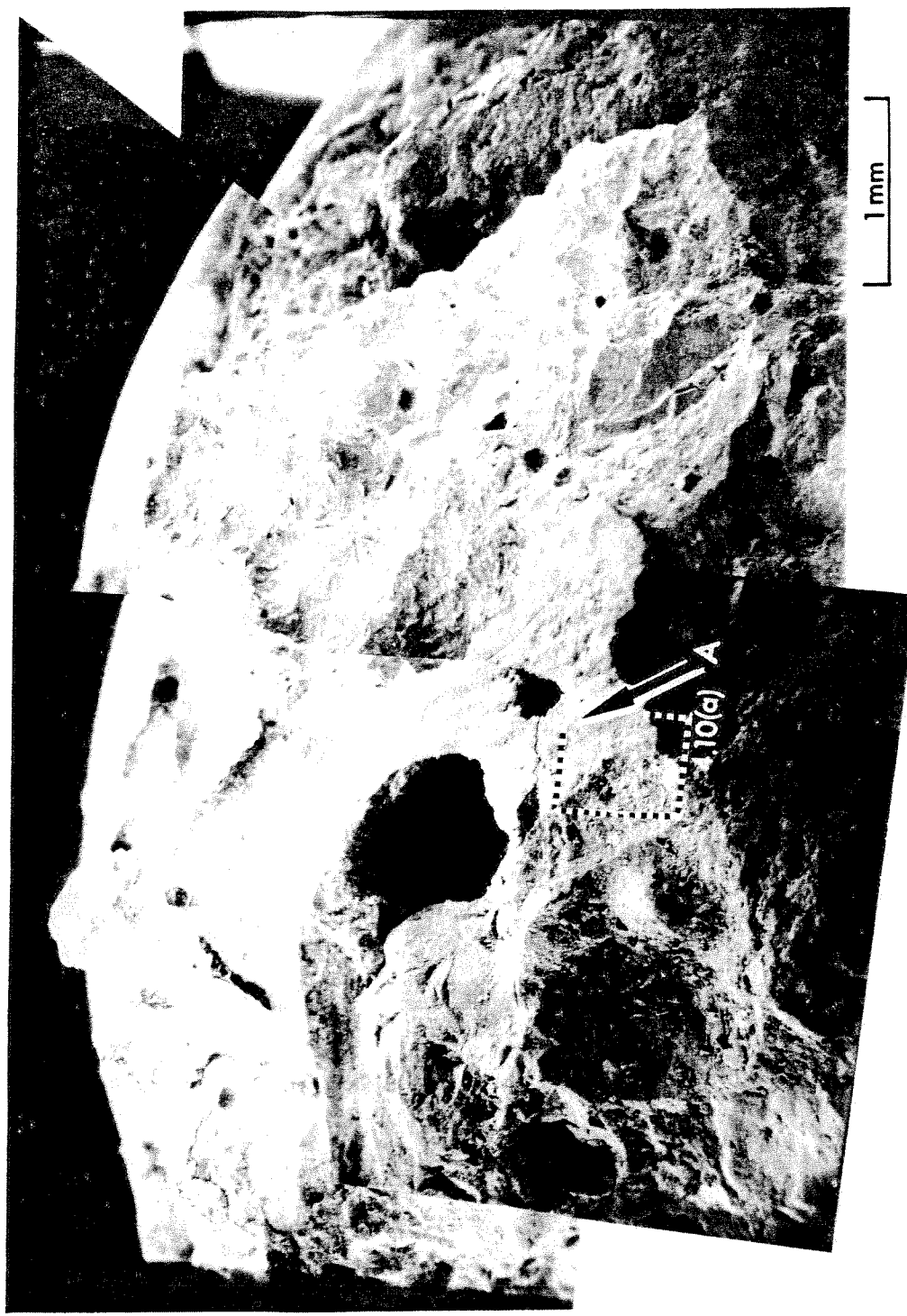
Figure 4.9. A mosaic of scanning electron micrographs showing the rough surface of mortar near the plain steel reinforcing bar when CrO_3 was not used. The small area marked A and several other areas of similar appearance were in contact with the surface of the steel. The many voids were caused by the evolution of hydrogen at the surface of the steel.
