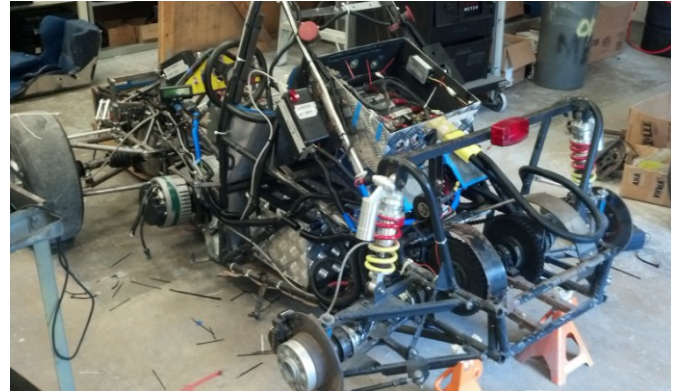
Fig. 1. Gamma rear-wheel drive setup. Dual PMG-132 and independent rear axle control.
