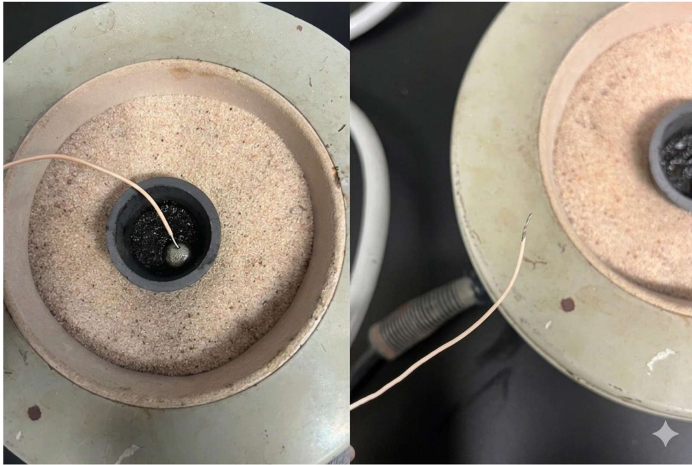
Figure 6. Solder bath pre-tinning and final wire attachment process for electrical connection. Lead wires are dipped into a solder bath to form a thin and uniform coating prior to attachment.
