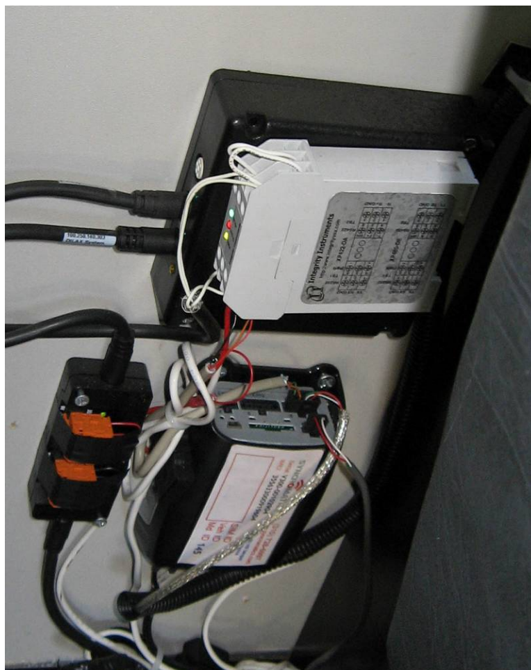
Figure 2 AVL Unit Installed on Bronco Express Shuttle Bus
