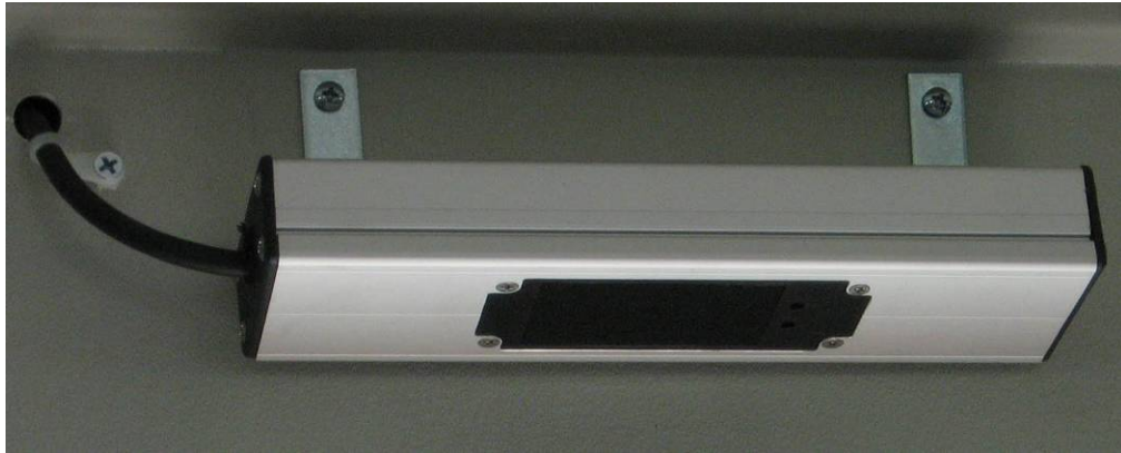
Figure 3 Automatic Passenger Counter Installed on Bronco Express Shuttle Bus
