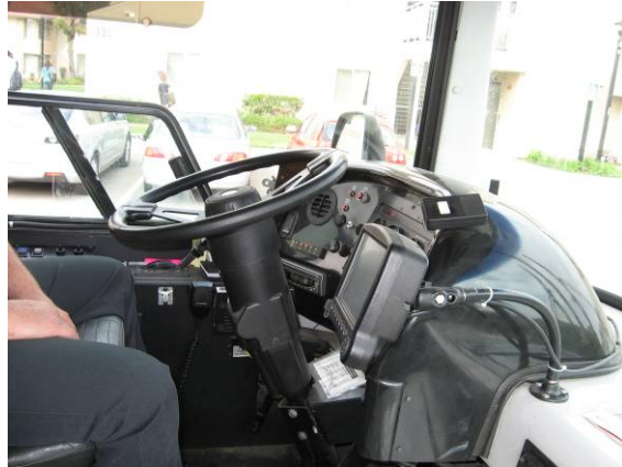
Figure 4 Mobile Data Terminal Installed on Bronco Express Shuttle Bus
