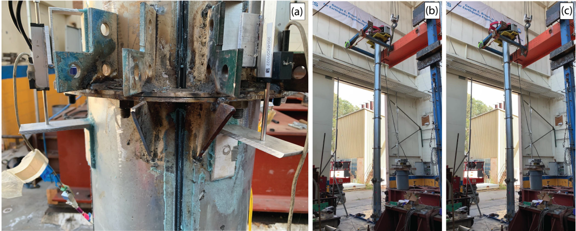
Figure 5.14: (a) Flange separation at the northern extent of the tower after the first forced resonance; the tower deflecting during forced vibration to the South (b) and North (c).
