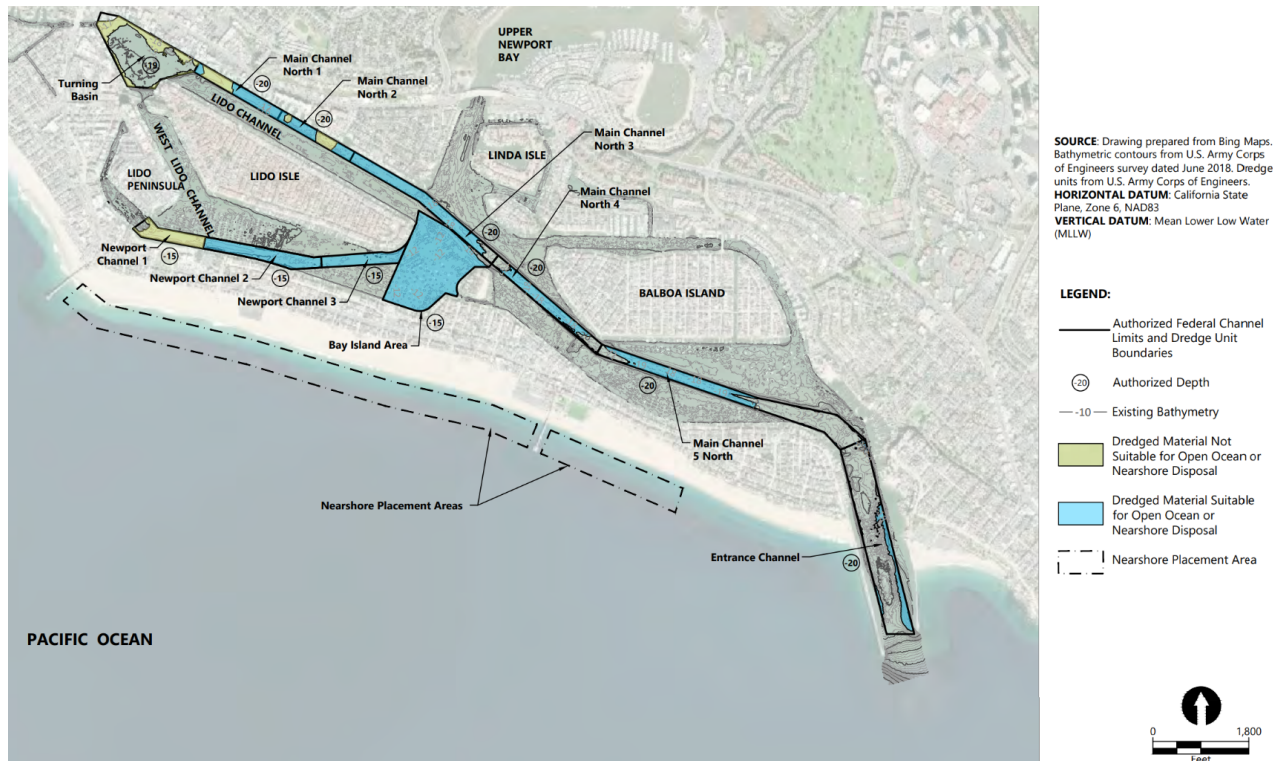
Figure 5: Federal Channels Maintenance Dredging Sediment Suitability Map, where the blue sections are the nine sites that are suitable for open ocean or nearshore disposal. 4
