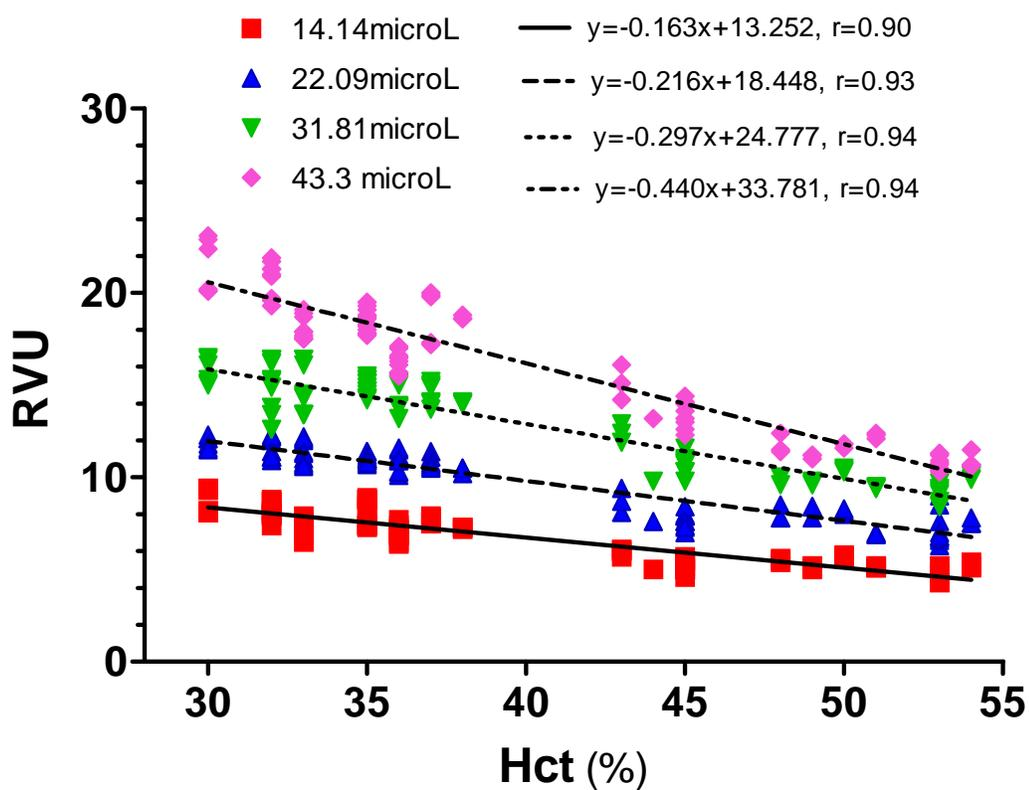
**Figure A2.1:** Linear regression of systemic hematocrit and blood conductance (RVU) in each known-volume cylinder. This calibration chart was created using our previous experiments (pooling data) in 20 blood samples for each cuvette.
