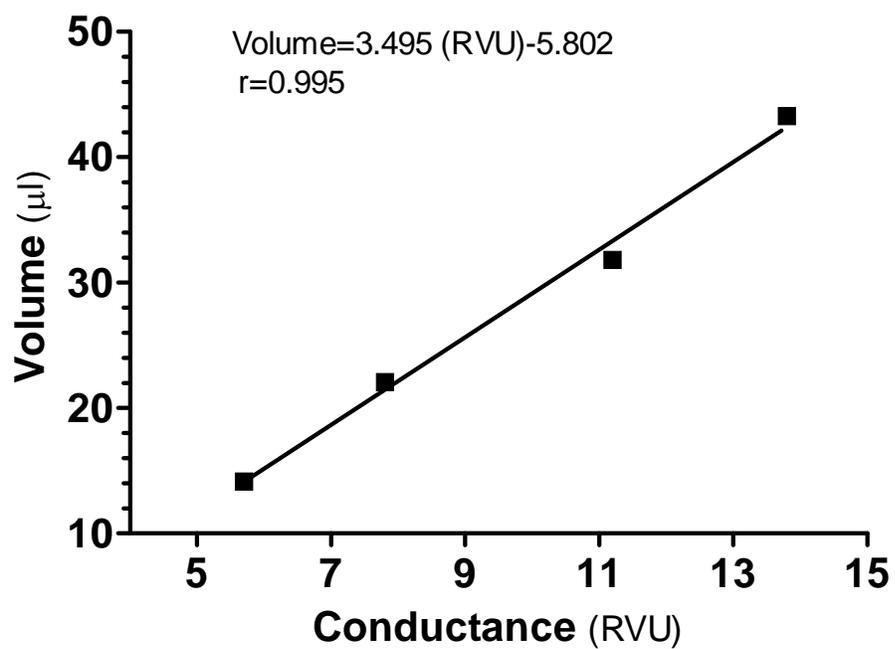
**Figure A2.2:** Linear regression of blood calibration from blood conductance (RVU) to actual volume (µl) in each known-volume cylindrical cuvette.
