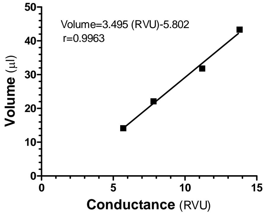
**Figure 3.1:** Linear regression of blood calibration from blood conductance (RVU) to real volume (µl) in each known-volume cylinder.
