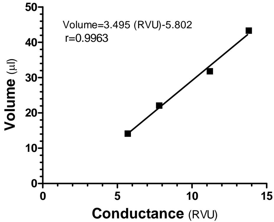
**Figure 2.1:** Linear regression of blood calibration from blood conductance (RVU) to actual volume (µl) in each known-volume cylindrical cuvette.
