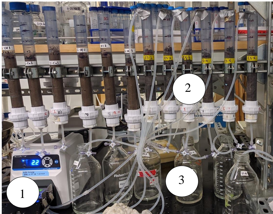
Figure 6-1: Experimental setup showing the pump (1) pumping stormwater into the columns (2), the effluents were then collected in the bottles (3).
