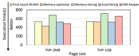
Figure 8.9: Evaluating HM-Keeper with different large page sizes. We use the SSSP application for evaluation.
