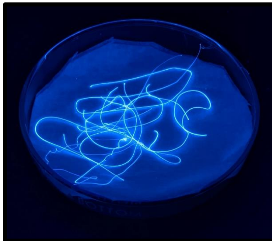
Figure 2.4 Fibers of PMMA doped with 4F9AC under illumination of a UV lamp, demonstrating the monomeric blue fluorescence.
