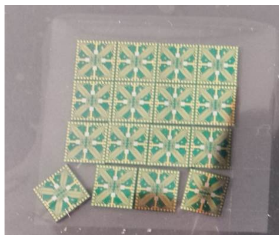
(b) Fabricated test sensors with spacings between working electrodes of 5 \mu\text{m} . Each chip contains a 4x4 array of IDE sensors as depicted in figure 1.6b
