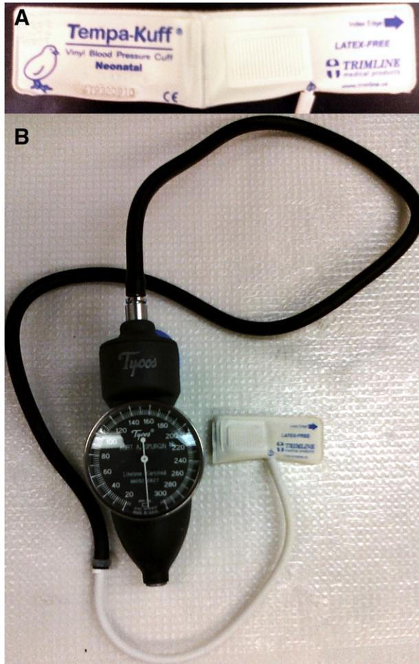
**Fig 1.** Apparatus used for applying calibrated massage therapy to rodents was developed using a modified neonatal blood pressure cuff. A neonatal blood pressure cuff (Trimline Tempa-Kuff, size 1) was modified via a midline cut that retained only the inflatable bladder (A). The neonatal cuff was attached to a standard clinical aneroid gauge (Tyco) via Luer connector (B).
