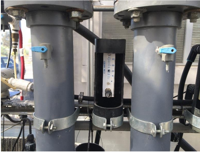
Figure B-2 Inlet samples were collected at the Inlet ports. Outlet rotameters were set at 20 mL min -1 .
