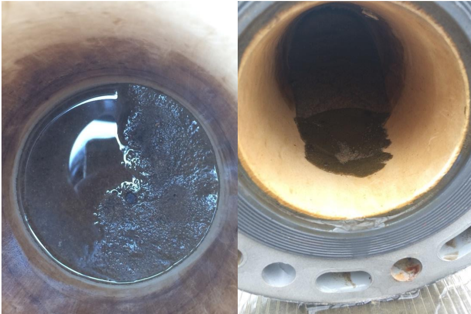
Figure B-5 Red biofilm layer formed on top of the sand columns after the first maintenance event (Day 20). Thick green gelatinous biofilm layer developed after 60 days of the project.
