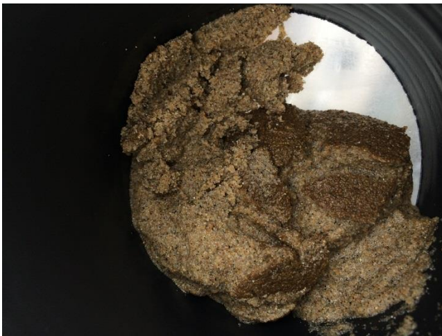
Figure B-6 Red crusty biofilm layer developed after first maintenance day.
