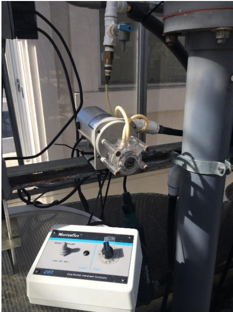
Figure B-4 Peristaltic pump controller limited the flow rate to the system at 120 \text{ mL min}^{-1} .
