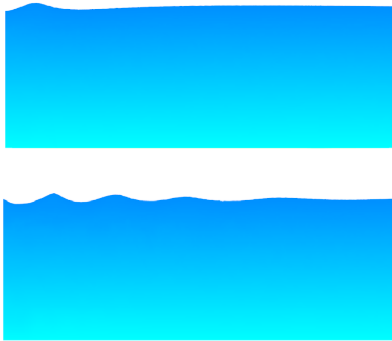
Figure 6.39: Two numerically generated wave conditions used for floating wind-turbine FSI simulations. Top profile corresponds to the Wave I case, while bottom profile corresponds to the Wave II case
