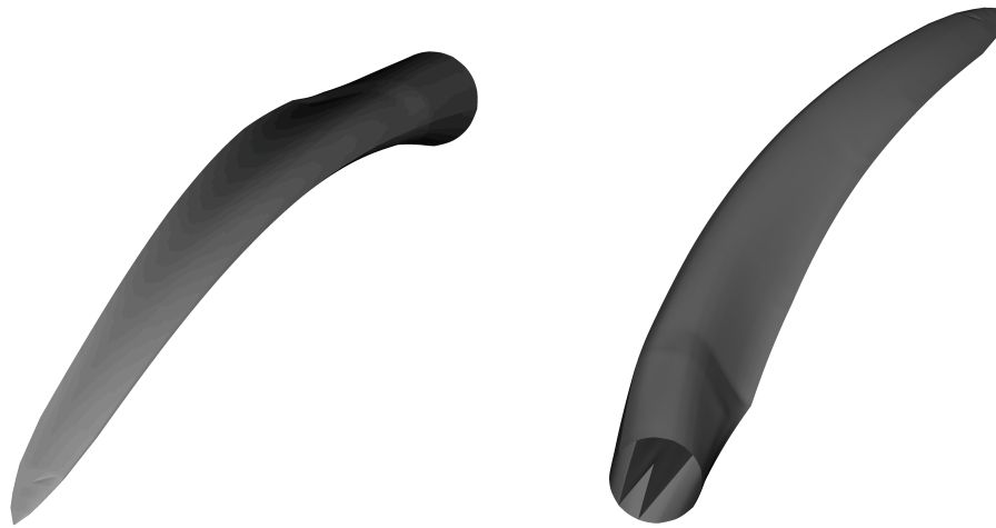
Figure 6.32: Eigenmodes of SNL 100-00 blade. Left: 1st bending mode; Right: 1st edgewise mode
