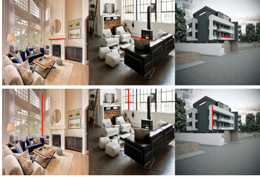
Figure 5.4: Line entity representation. For each row, we show how a same line entity predicts line segments with same property in three different indoor/outdoor scenes. The top line entity is specialized for horizontal line segments in the middle of the figure, and the bottom one prefers to predict vertical line segments with a various range of lengths.
